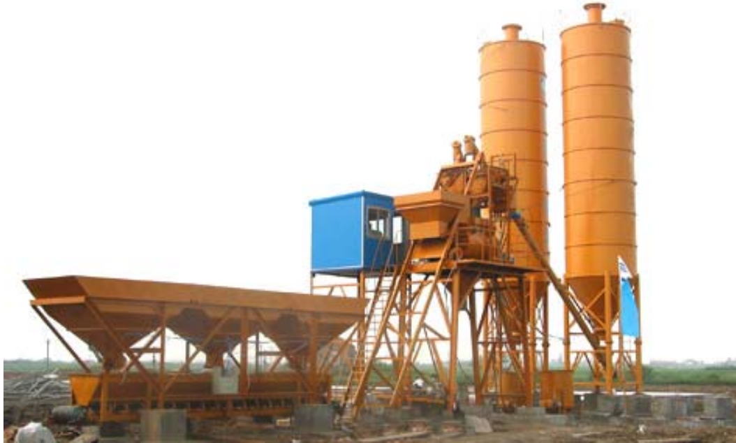
HZS35J Static concrete mixing plant
